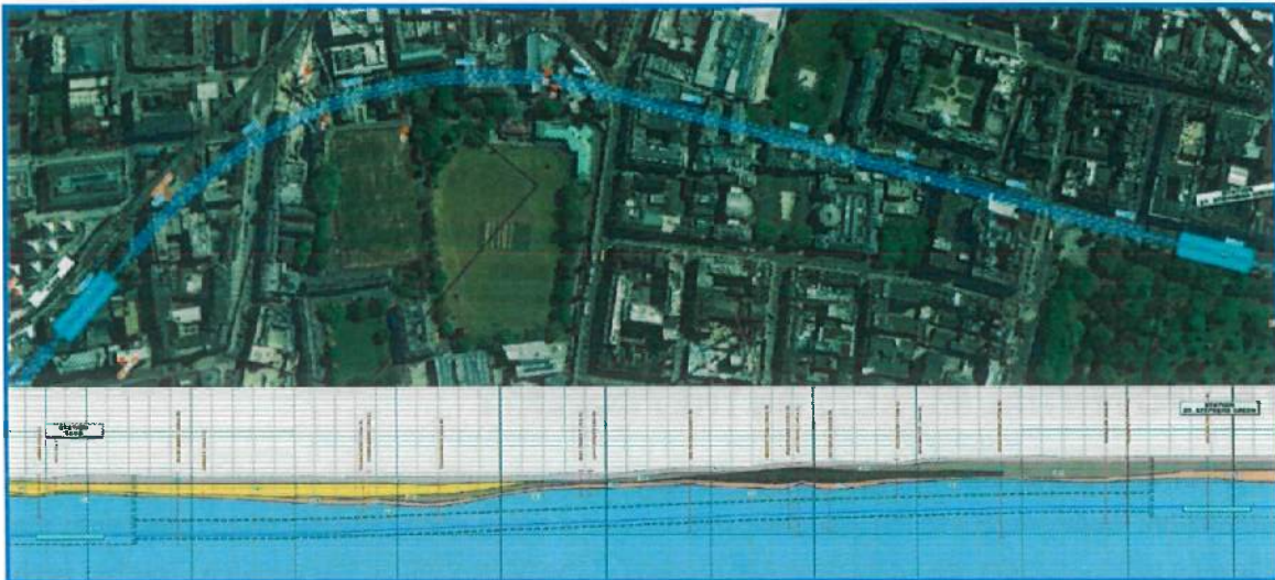
Figure 16. Geographical Section (ref. A5.13, Diagram 3.13: Geologic Profile for TBM Drive C8- Tara Station to St. Stephen's Green)
